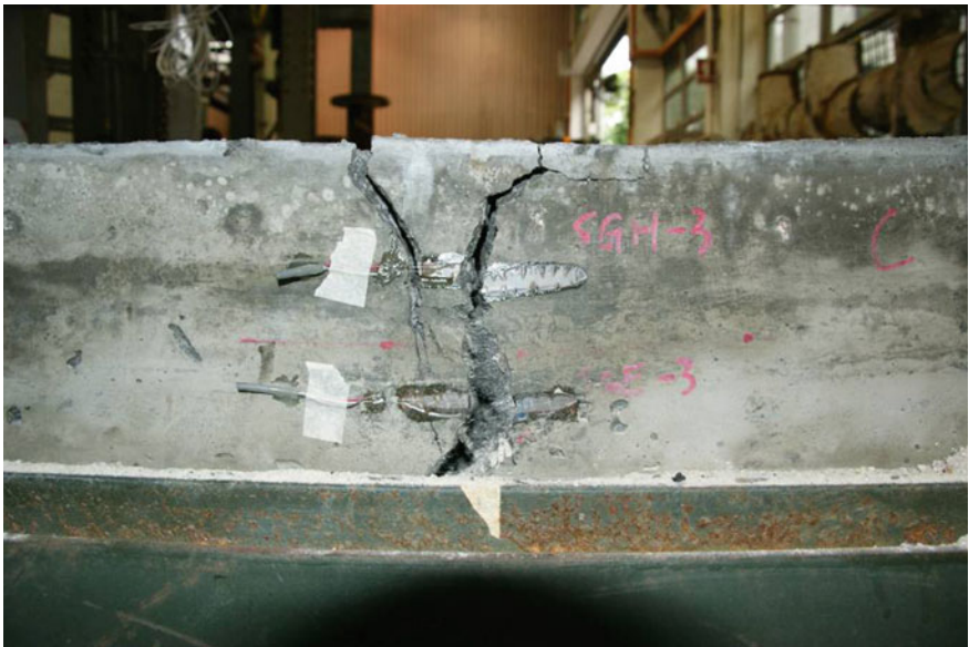
Fig. 2.40 Side 2 profile of Sample D after second impact
