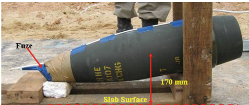
Fig. 3.1 M107 Placement on Slab
