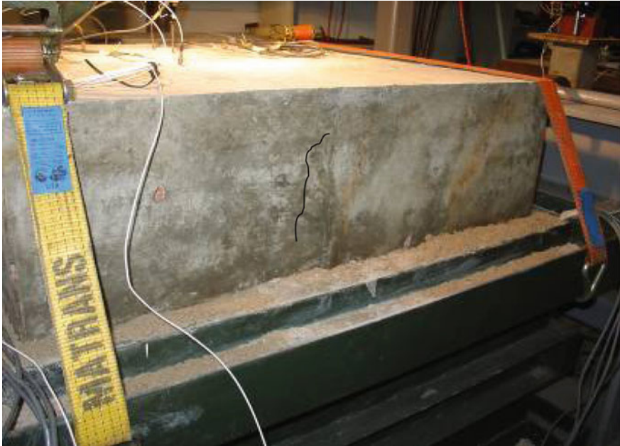
Fig. 2.13 Crack Propagation in Sample A after first impact
