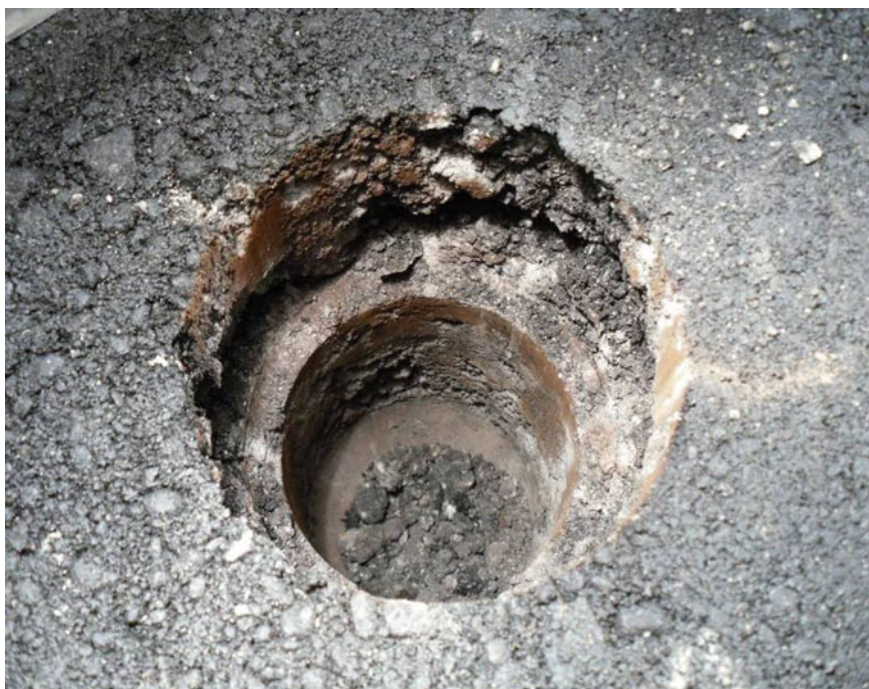
Fig. 2.23 Crater of Sample B after second impact
