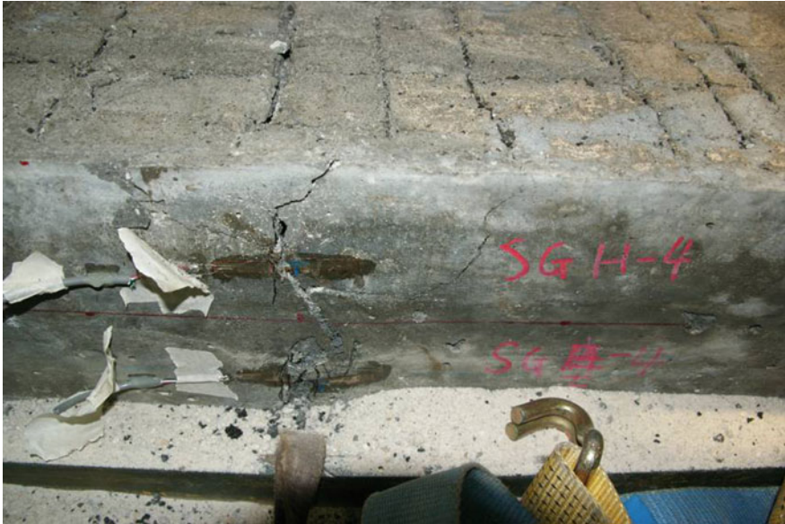
Fig. 2.39 Side 1 profile of Sample D after second impact
