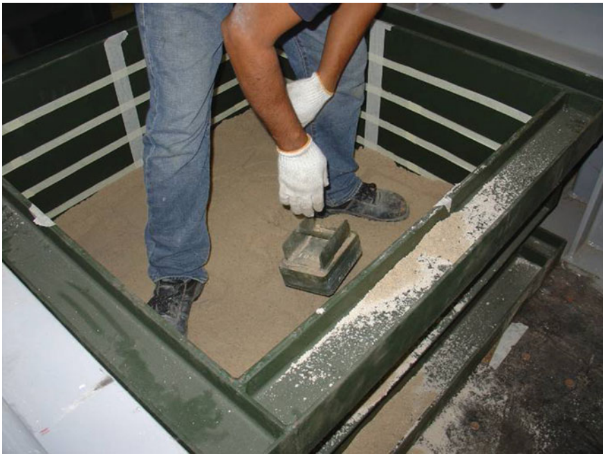
Fig. 2.5 Compacting of sand in steel strong box
