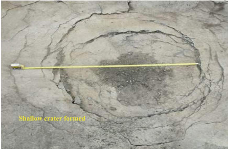
Fig. 3.38 Detail of crater for the Slab 2
