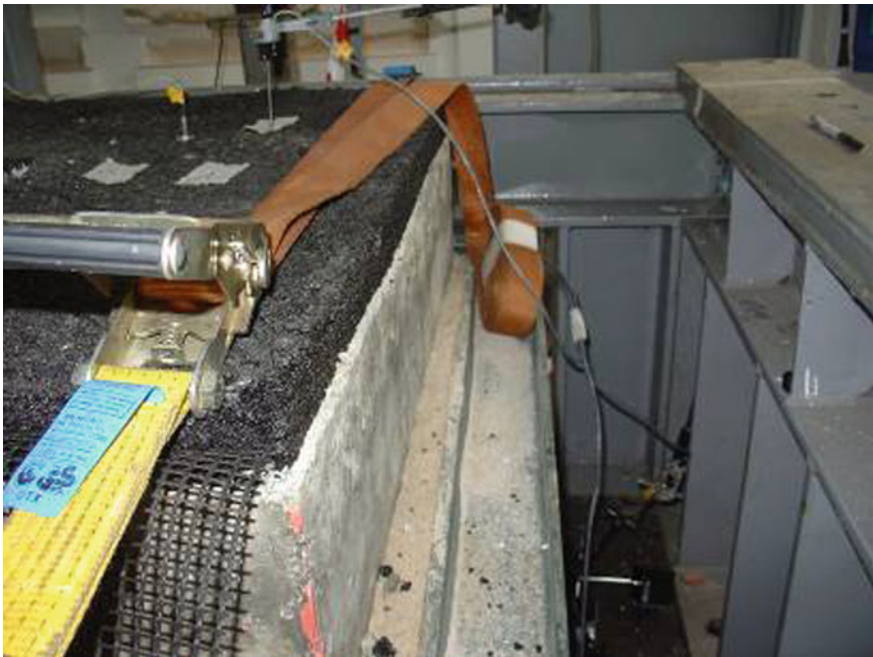
Fig. 2.31 Shift of asphalt layer in Sample C after second impact
