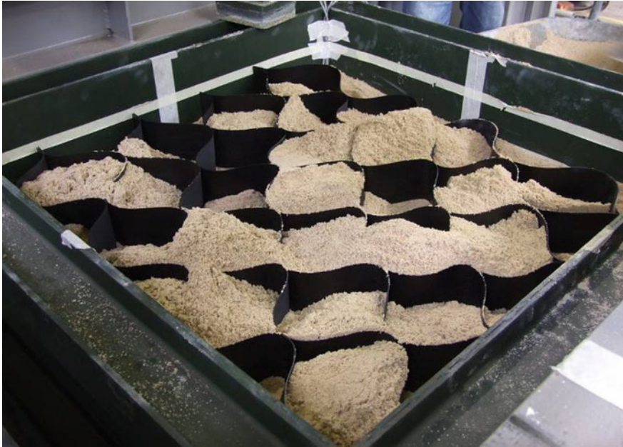
Fig. 2.6 Geocell used to reinforce the sand in the steel strong box
