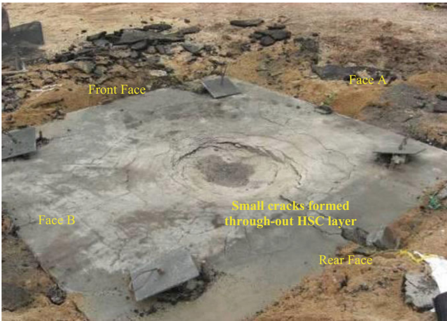
Fig. 3.37 Crater details for the Slab 2 after removal of asphalt layer
