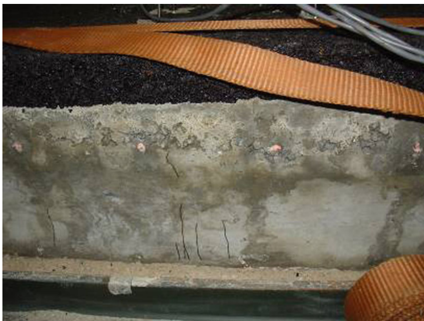
Fig. 2.27 Side profile of Sample C after first impact
