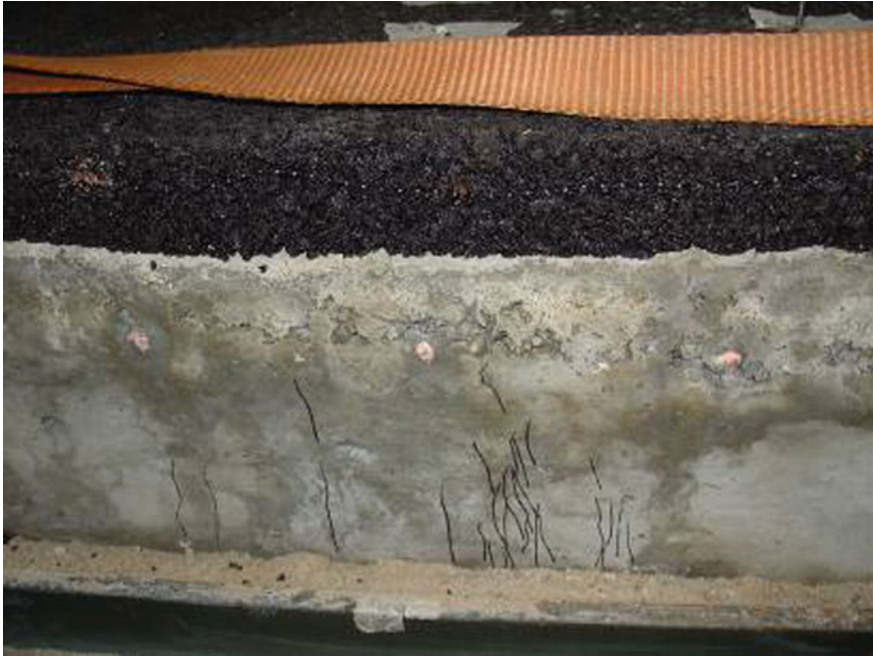
Fig. 2.30 Side profile of Sample C after second impact
